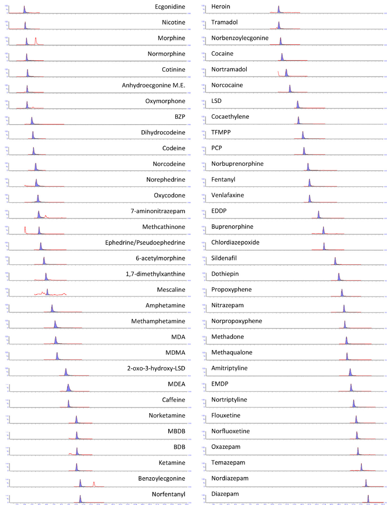
Fig. 1. UPLC–MS/MS separations for compounds spiked into WWTP influent before extraction (concentration, 500 ng L -1 ).
